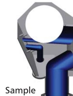
Sample outlet features a reducing ferrule (.75" connection to a .5" port) to maximize drainability of the small diameter port.
